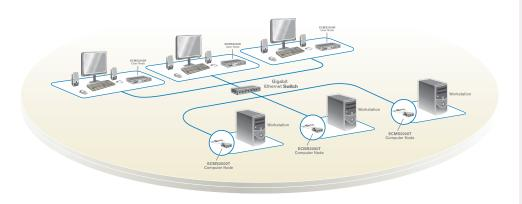
The Emerge ECMS2000 digital workstation extender includes computer nodes and user nodes that can be interconnected in a point-to-point configuration at Gigabit Ethernet rates using IP protocols over a single UTP cable. The ECMS2000 extender makes it possible to back-rack digital workstations without impact to post-production operations.
