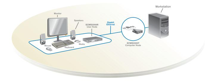
The Emerge ECMS2000 digital workstation extender provides hardware-based extension for digital/analog video, USB keyboard and mouse, USB media, and audio signals.
